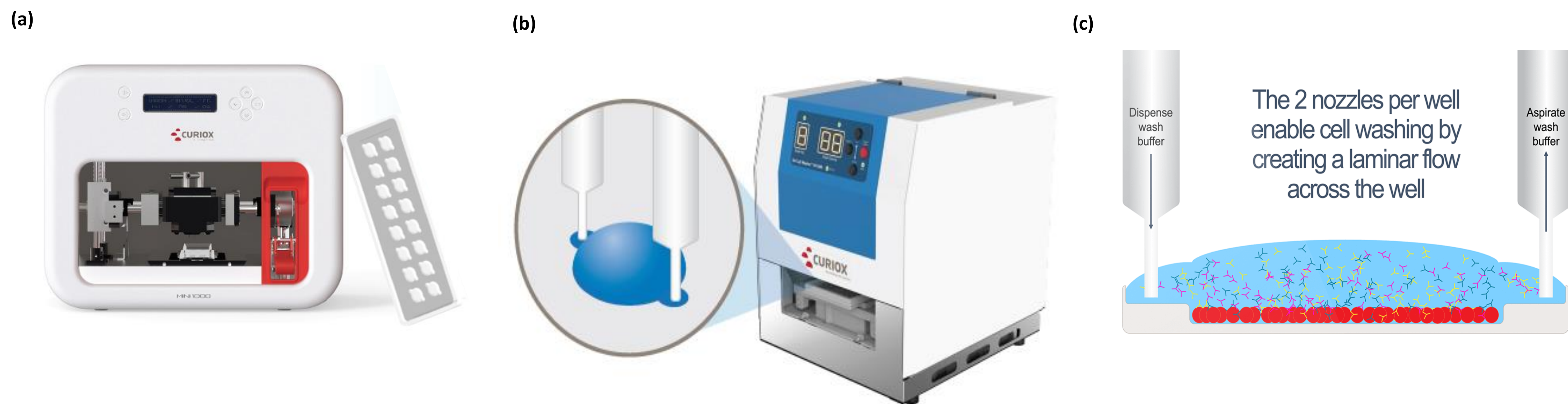
Fig 1 Curiox's centrifuge-less cell preparation platform is enabled by our wall-less plate and laminar flow washer .
